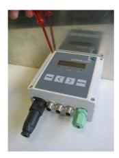
Disconnect the voltage of the RMA-POWER-BOX 107 and secure it against being switched on again. Open the four mounting bolts of the cover as shown.
