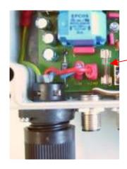
Remove defective fuses and replace with new fuses. (I=4A T)
